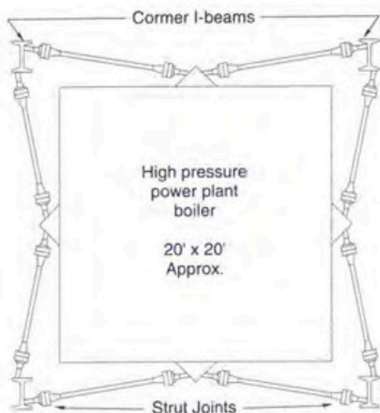
Fig.8 — Engineers needed to brace a 60ft (18.3m) high power plant boiler against wind sway and allow for downward thermal expansion of the boiler and its integral furnace. The boiler is supported by hanging from the top, within four I-beam corner columns. Eight Flexible Struts, in opposite pairs at 35ft (10.7m) and 50ft (15.3m) were used to meet these requirements efficiently and economically. The use of eight struts allowed the construction of a lighter steel structure at the anchor points.
