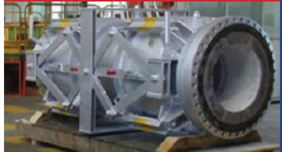
Cold Wall Standpipe Expansion Joint with Pantograph Hardware
