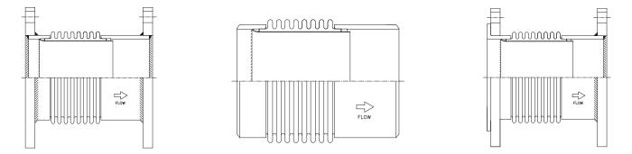
Flanges: Flat face carbon steel made from ASME A-36 plate. Outside diameter and drilling per ASME/ANSI B16.5. Table 2 designs—150 lb. drilling, Table 3 designs—300 lb. drilling.
