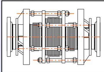
This expansion joint is another unique design that absorbs axial, lateral and angular movements while eliminating pressure thrust loads on the piping and without a change in direction of the piping. Through the use of a balancing bellows
